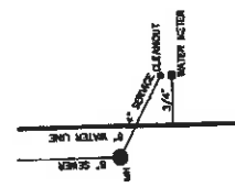
TYPICAL WATER & SEWER SERVICE
