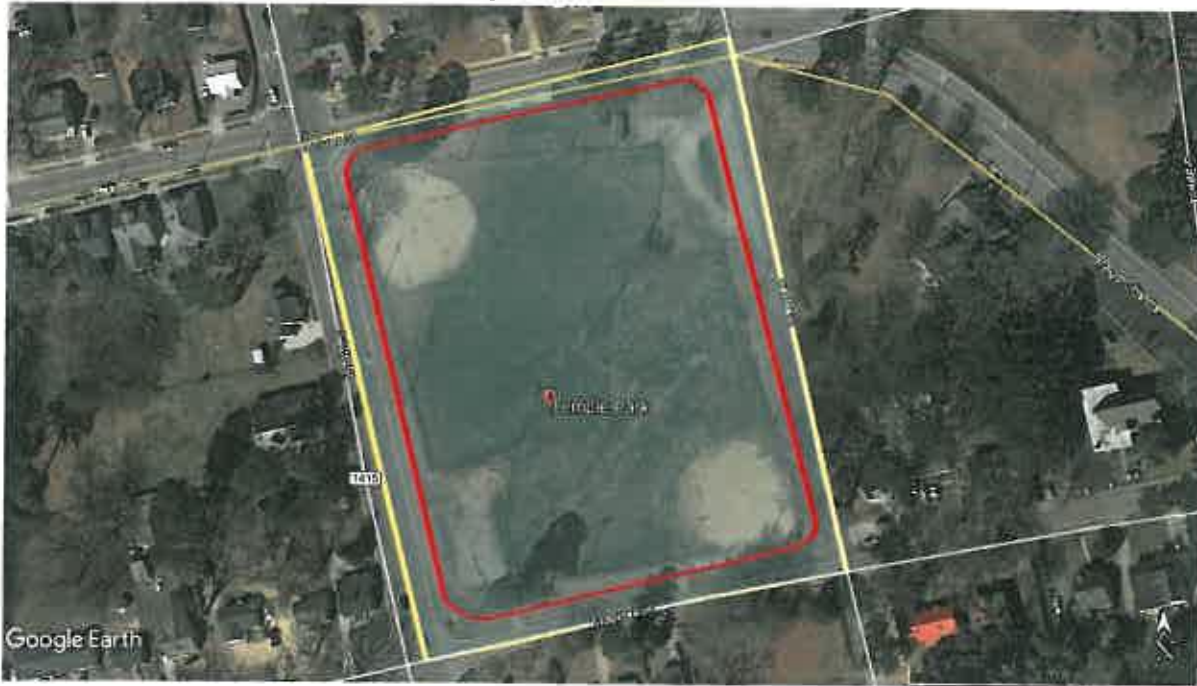
Red Outline: Boundary Survey limits Yellow Area: Phase I Topographic Survey limits
